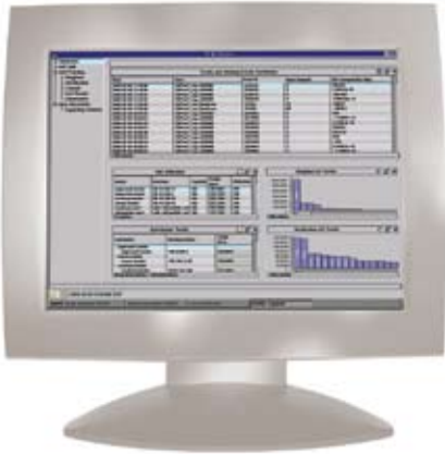
Traffic Summary: Traffic Explorer's summary report provides an overview of key traffic data including a list of all routing events showing the impact on traffic, network-wide link utilizations and BGP-related traffic statistics
